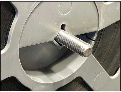
For 16mm reels of film, simply slide the reel onto the left source spindle as shown. Film should feed from the left side of the reel
