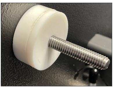
The purpose of the spacer is to position the source reel so that the film does not rub against the reel as it is being scanned. This spacer will work for most all reels. If needed, washers from a hardware store can be used to suppliment or replace this spacer for better 8mm reel alignment.
