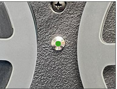
After blinking red, the light will then blink green. When scanning, the light will be solid green and not blinking.
