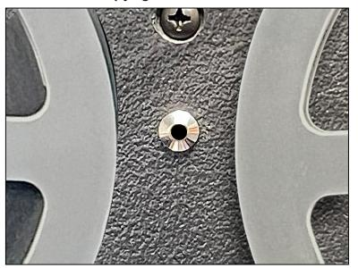
When the Ethernet cable is not plugged into the PC, this pilot light will be off.
