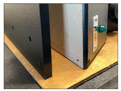
Lay the unit on its side on a non-marring surface. Align the plate with the bottom of the unit. It does not matter which end of the plate faces front as the plate is symmetrical.
