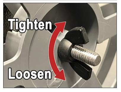
The take up reel is held in place with a simple wing nut. There is no need to over-tighten the wing nut as its job is merely to keep the reel in place.
