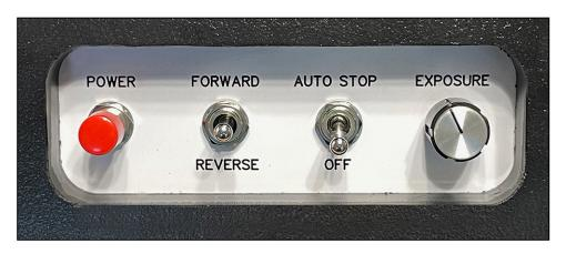
The controls are pretty simple. The **Red Buttom** turns power on and off for the entire unit. **Foward** and **Reverse** has a center stop position. If activated, the **AutoStop** switch will stop the unit after 15 seconds if frames are no longer being captured due to misalignment of the LightPin sensor, end of reel, or if film breaks or jams. The **Exposure** knob is used during manual exposure and can help to find tune the software's auto exposure function.
