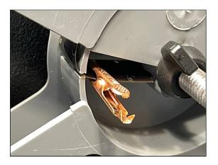
The accessory kit includes two film clips that are a handy way to secure the end of the film to the reel as shown. Juste remember to remove the clips when you are finished scanning about about to rewind the roll.
