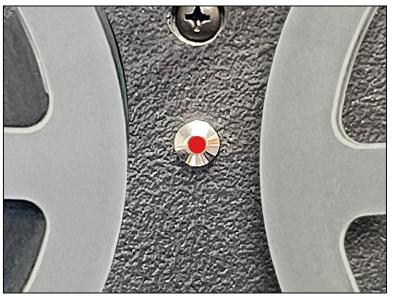
When the Ethernet cable is plugged into the scanner with the software active, this light will start to blink red.
