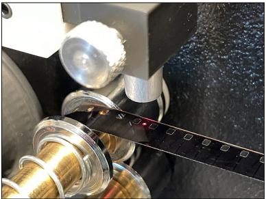
Once focus on the LightPin Sensor is achieved, move the red dot to the middle of the sprocket hole path.
