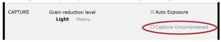
RetroScan can capture in both compressed or uncompressed formats. The default setting is for compressed, where every frame is stored as a hi-resolution JPEG. Checking the box will allow you to capture uncompressed, where each frame is a BMP. Please note that capturing uncompressed requires an increased amount of drive space and speed.
