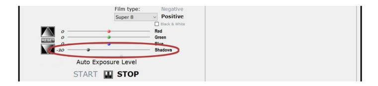
Shadow Detail is normally at -20 but can also be changed to suit the needs of the footage. In general, these settings are a good starting point that will work for Auto Exposure on most home movies with moderate over and under exposure. For radically under exposed or over exposed films, you may have better results using manual exposure.
