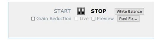
PREVIEW can be used to see how your film will look without actually capturing it to your harddrive. This can be used whether the film is stationary or running. Just be aware that, if the film is not running, then the film isn't under tension and the image may not reflect accurate focus. Typically, it is best to adjust focus while the film is running.
