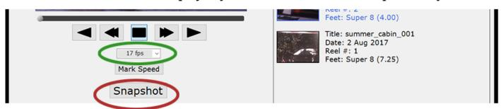
If you see a particular frame that you would like to use for an enlargement or perhaps a DVD or BluRay cover, you can click on the "Snapshot" button and the software will output a high resolution still frame which can be found in the Export folder. To see the movie played at a variety of speeds, simply use the speed drop down menu.
