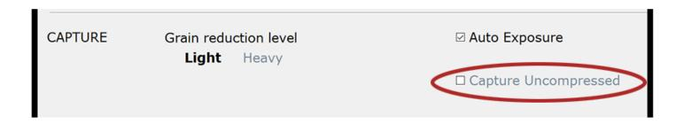
RetroScan can capture in both compressed or uncompressed formats. The default setting is for compressed, where every frame is stored as a hi-resolution JPEG. Checking the box will allow you to capture uncompressed, where each frame is a BMP. Please note that capturing uncompressed requires an increased amount of drive space and speed.
